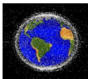
Figure 2: Low Earth orbit, the region of space within 2,000 km of the Earth's surface, is the most concentrated area for orbital debris. Photo courtesy of NASA ODPO
