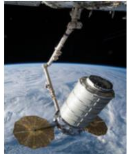
Figure 1: The Orbital ATK space freighter is slowly maneuvered by the Canadarm2 robotic arm toward the Unity module for installation on the International Space Station to resupply the Expedition 55 crew.
