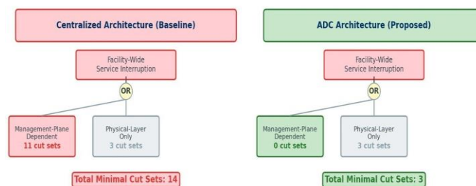
Fig. 3: FTA cut set comparison: centralized (14 cut sets, 11 management-dependent) vs. ADC (3 physical-layer cut sets only).
